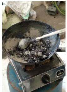
Fig 1: Mixing of Coated Aggregate and CRMB
