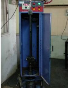
Fig 2 Automatic Marshall Compactor
